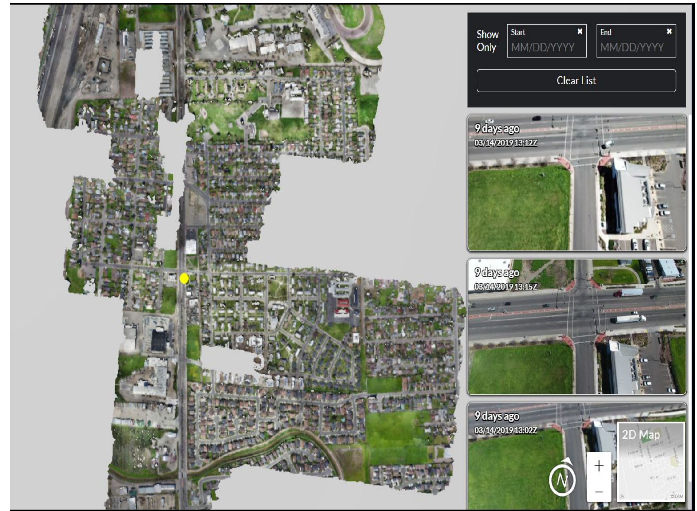
Figure 4.8 is an example of the 3D map generated from the collected footage. Users can also select a point on the 3D map to view video footage from multiple angles of an area of interest.
